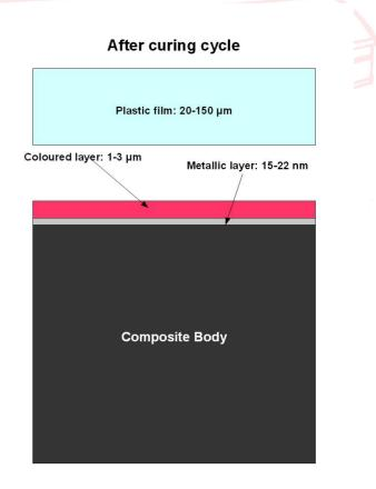
left on the composite's structure to form an additional protection to the surface. Please we aware that also the application, the manufacturing method has been patented.
